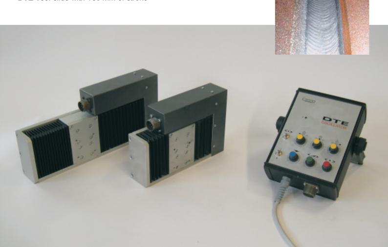
DTE is a linear oscillator with electronic motion reverse
