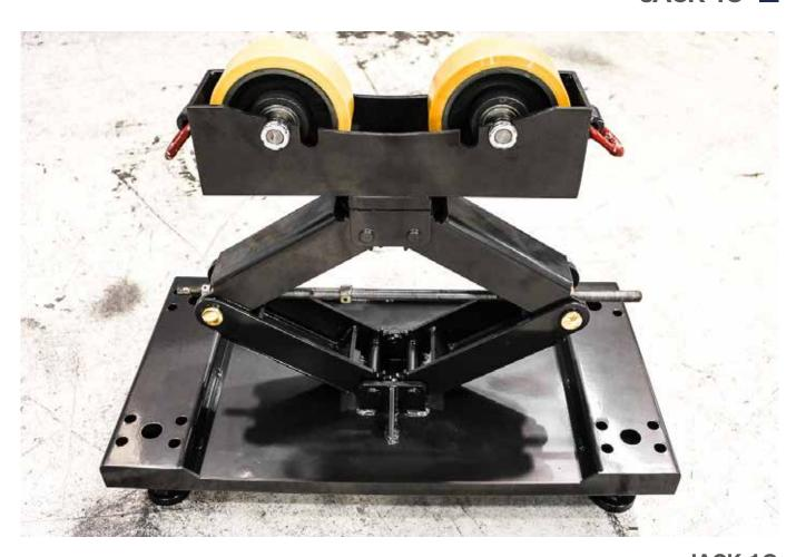
**JACK 10** Stationary execution, with four levelling shoes. The sketch hereunder shows JACK 10 supporting a pipe in combination with positioner JODA20
