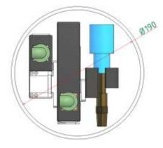
to correct the torch position inside small pipes, in circumferential position or longitudinal. please note also as in the 2 exemples change also the connectors position
