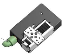
2 axis model, in this drawing the connectors are on the top side
