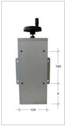
SM BIG is made of aluminium plates and profiles, it moves on linear precision ball guides driven by trapezoidal screw. Payload 60 kg at 0.4 m from face plate allows to combine it with other slides and makes it suitable for heavy duty jobs and SAW.
