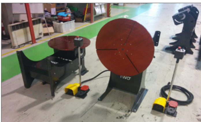
Special version with increased table up to \varnothing 650 mm and supporting feet in order to bring the table to a low ground height.
