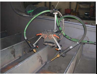
A sample of application on flat panel: thickness 20 mm and height 400 mm
