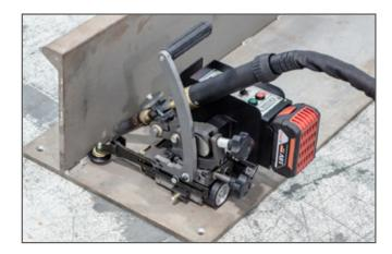
Corner inner welding with drive wheels on the horizontal plate of the workpiece.
