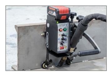
Corner outer welding with drive wheels on the vertical plate of the workpiece.
