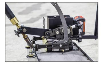
Corner outer welding with drive wheels on the horizontal plate of the workpiece.
