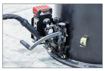
Corner outer welding with drive wheels on the circular wall of the workpiece.
