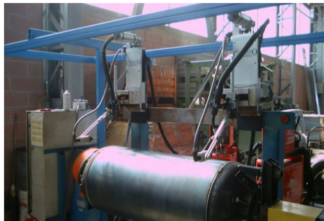
IG MD 250/2 MIG Vessel welding In this application the vertical slide is connected on the carriage, so all the slide move Up and Down
