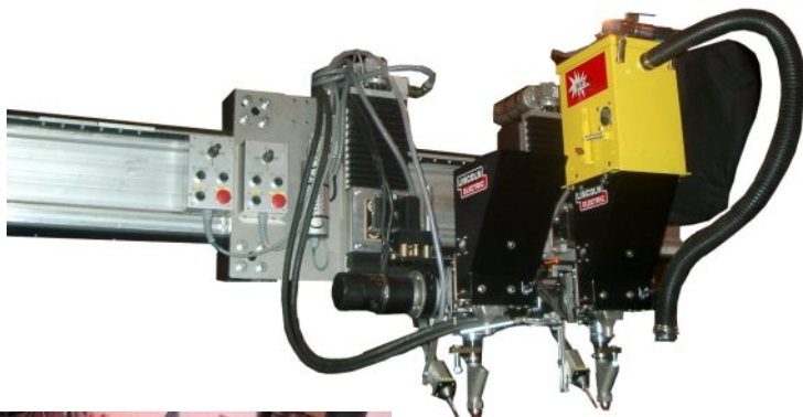
SAW seam tracker installed on a motorized carriage and a vertical slides.
