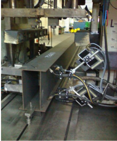
IG LT 80/2 Box beam welding Mig process with 2 head at the same time
