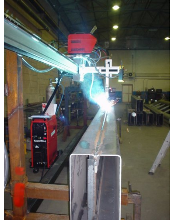
IG MD 250/2 MIG Vessel welding In this application the vertical slide is connected on the carriage, so all the slide move Up and Down
