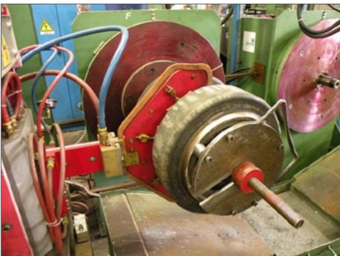
pre-heating joint prior to automatic welding.
