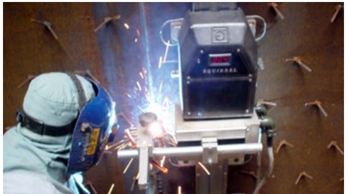
Squirrel with oscillator for vertical welding
