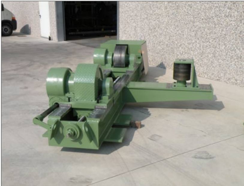
Steered anti-drift, manual or automatic Example of manually operated anti-drift: the system is applied to the idle unit, whose wheels are steered (2) to generate contrast to the drift of the workpiece.
