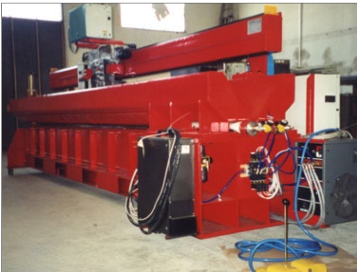
Horizontal for inner welding of pipes or flat sheet metal
