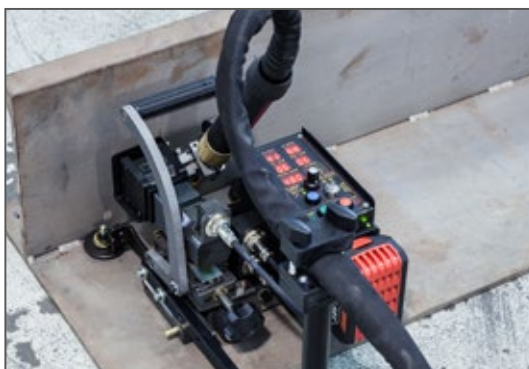
Corner inner welding with drive wheels on the horizontal plate of the workpiece.
