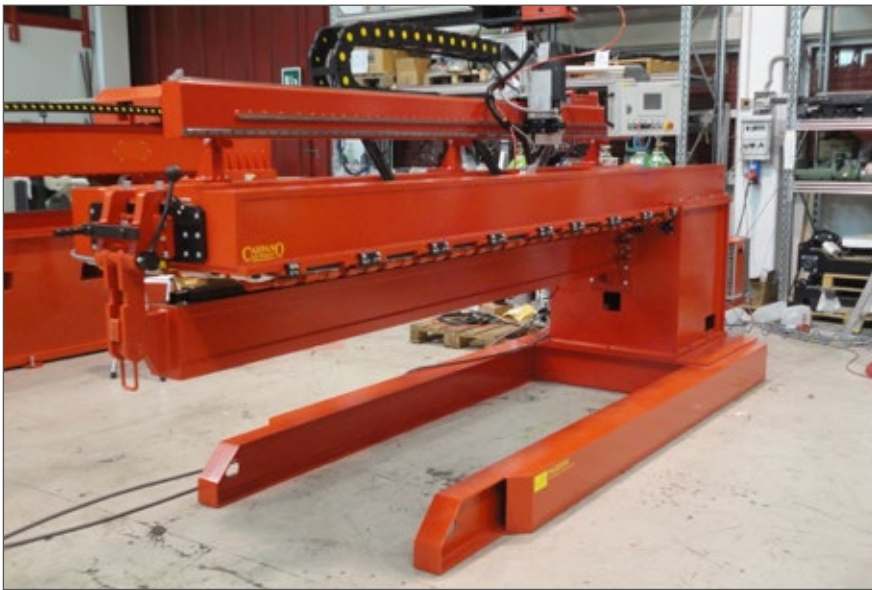
Horizontal for inner welding of pipes or flat sheet metal
