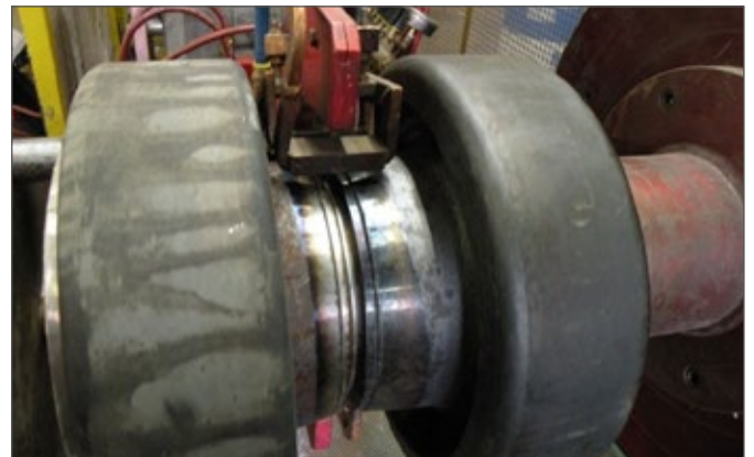
pre-heating joint prior to automatic welding.
