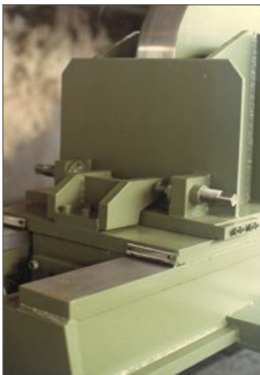
Steered anti-drift, manual or automatic Example of manually operated anti-drift: the system is applied to the idle unit, whose wheels are steered (2) to generate contrast to the drift of the workpiece.
