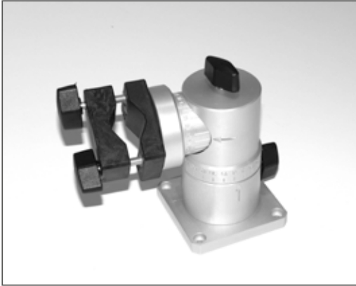
TWIN 2-axis rotating torch holder, 360° on both axis, with angle indication, clamp for torch \varnothing 18 to \varnothing 40 mm and brake to fixit in the right position.
